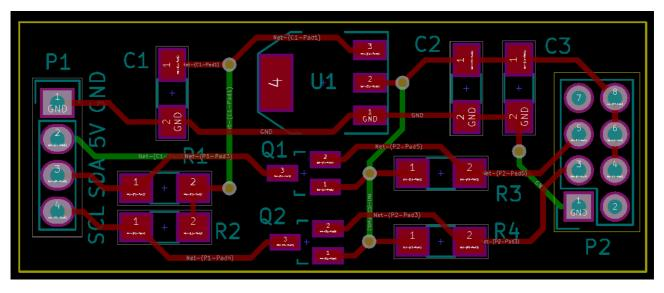
You simply connect the Nixie Time Module to the existing I2C interface on the clock. The pins on P1 line up 1 to 1 with the pins on the Clock Module. You can either connect directly, or using flying leads.
