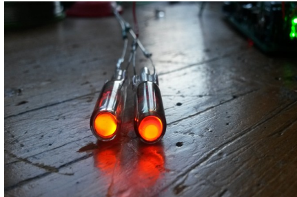
Driving 2 neons from the “Tick” circuit
