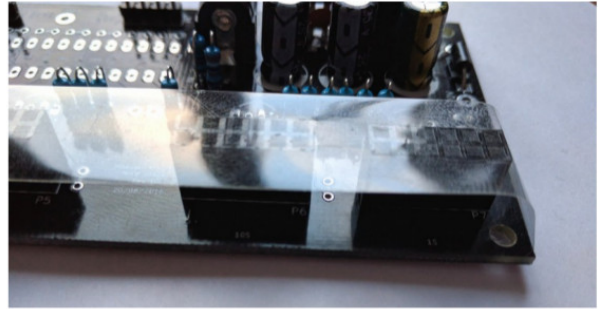
Tape the sockets in place
