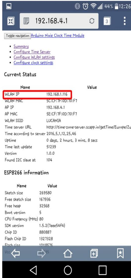
The screenshot shows the configuration page for an "Arduino Nixie Clock Time Module". At the top, the IP address 192.168.4.1 is displayed in a search bar. Below the navigation menu, the "Current Status" section contains a table with the following data:
